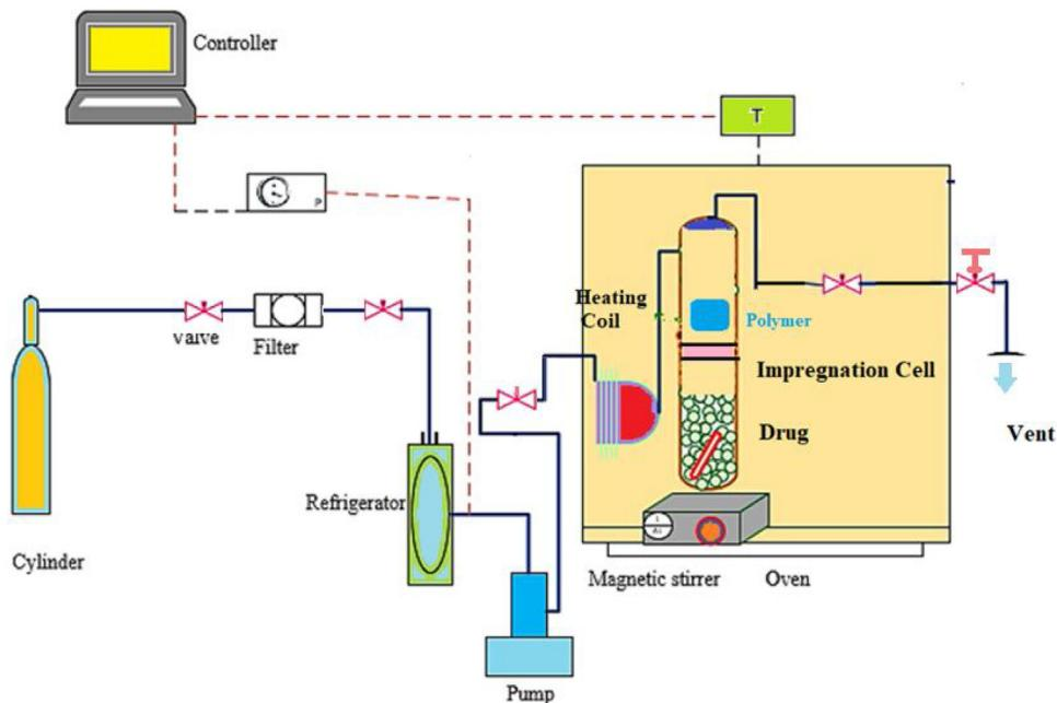
**Fig. 2.** Experimental apparatus of supercritical CO<sub>2</sub> impregnation.
