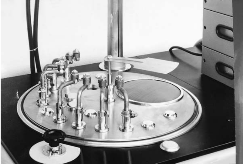
Figure 9.4. The base-plate of a thin-film coating plant showing the electrodes and the shutter used for terminating the layers.
