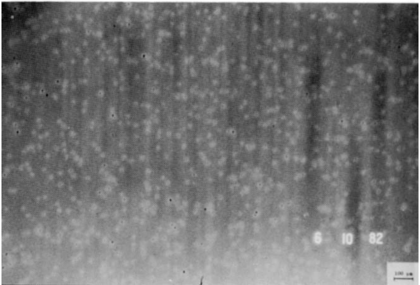
Figure 10.8. Moisture-penetration patterns in a multilayer of zirconium dioxide and silicon dioxide. The photographs were taken immediately after removal from the coating chamber. The wavelength for the upper photograph was 543 nm, and that for the lower 553 nm. (After Lee [29].)
