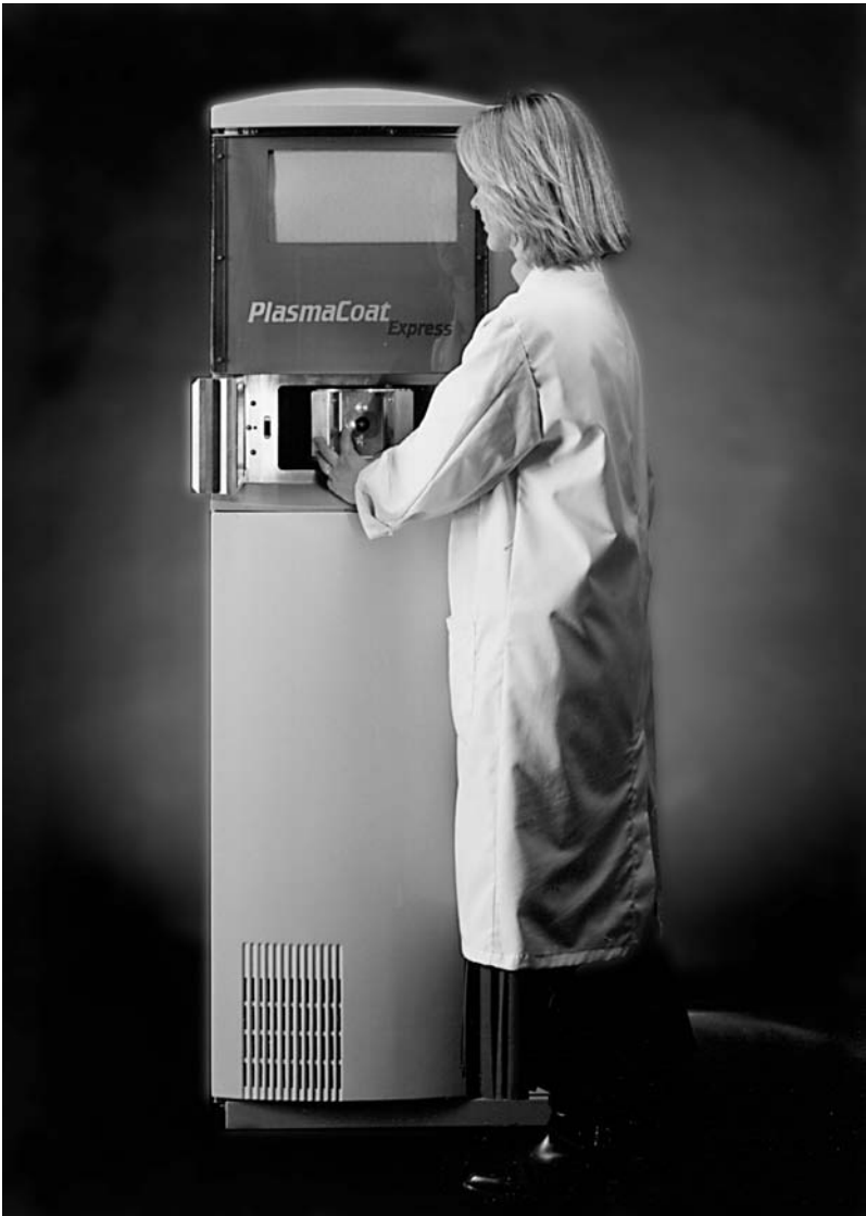
Figure 9.11. The Plasmacoat is a small machine intended principally for the coating of spectacle lenses but it can also be used for small batches of other types of coating. The process is one of reactive sputtering and the operation is entirely automatic. The coating chamber is permanently under vacuum. For loading, the substrate carrier drops down into the loading chamber leaving the coating chamber sealed off. The carrier can then be loaded through the access door. Once substrates are loaded the access door closes and the substrate carrier moves upwards back into the deposition chamber. (Courtesy of Applied Vision Ltd, Coalville, Leicestershire, England.)
