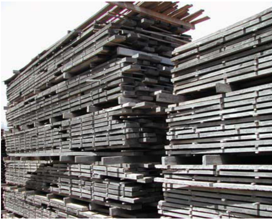
Fig. 4.10 Air seasoning of Jarrah wood in Western Australia
