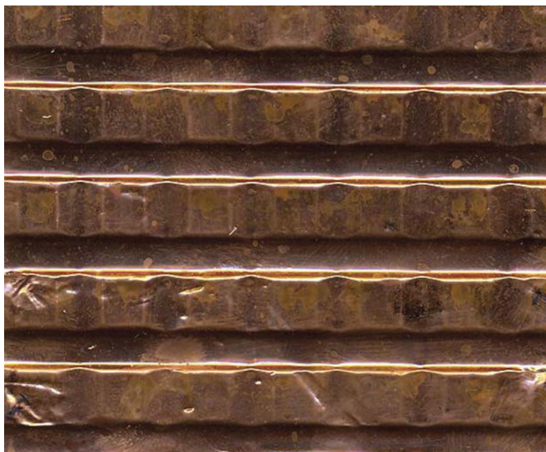
Fig. 6.4 Copper-faced bitumen membrane roofing
