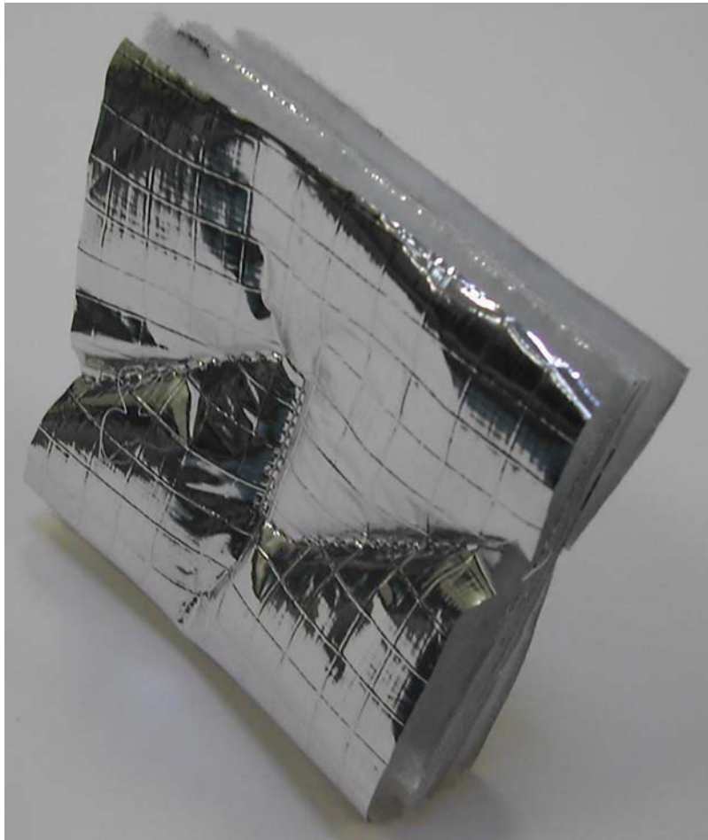
Fig. 13.4 Multi-layer aluminium foil insulation system
