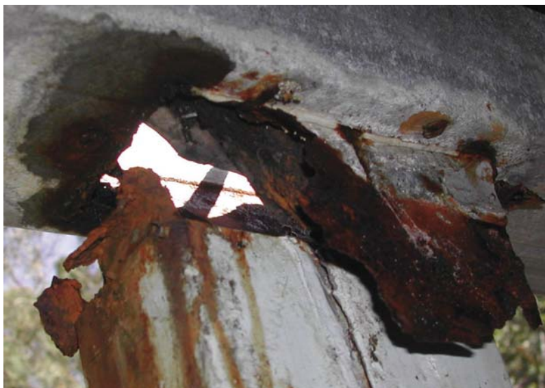
Fig. 5.37 Bimetallic corrosion between aluminium and steel
