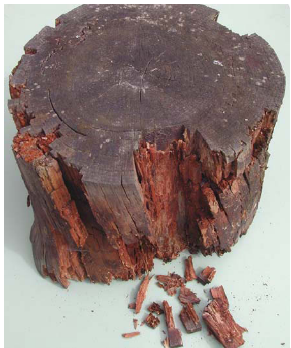
Fig. 4.21 Deterioration of sapwood timber illustrating the relative durability of heartwood over sapwood
