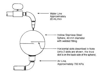
Note 1—Cut three horizontal air slots around circumference of hollow sphere using a  $0.20~\rm mm$  thick diamond lapidary saw covering  $120^{\circ}$  to  $150^{\circ}$  each and spaced approximately 5 mm apart. Air passing through these slots strikes the water (which is flowing over the outer surface of the sphere) to produce a spray.
