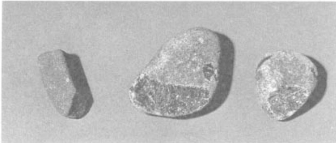
FIG. 5 Fractured Particle (Center) Flanked by Two Non-Fractured Particles (Chipped Only)
